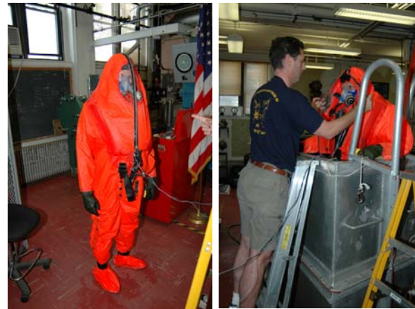
Fig.1: Rebreathing tests with the MK10 SEIE suit while unimmersed (left photo) and while immersed in a water tank (right photo). The right photo also shows the Genetex mask that was worn to permit measurement of metabolic gas exchange.
